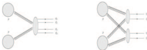
Fig. 3. – \Upsilon production diagrams for SPS (left) and DPS (right) irreducible backgrounds.
