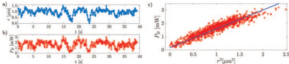
Fig. 2. – Displacement  $r$  from the equilibrium position of the particle (a) and optical power inside the ring cavity  $P_B$  (b) as a function of time  $t$  for 10 seconds of a 100 second trajectory.  $P_B$  as a function of  $r^2$  (c). The solid line in panel (c) is the fit curve to check the linearity of our data.
