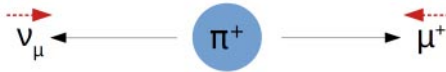
Fig. 2.: Decay of the positive pion in the rest frame of reference. The spin of the muon points toward the pion as the neutrino must be left-handed because of parity violation of the weak interaction.
