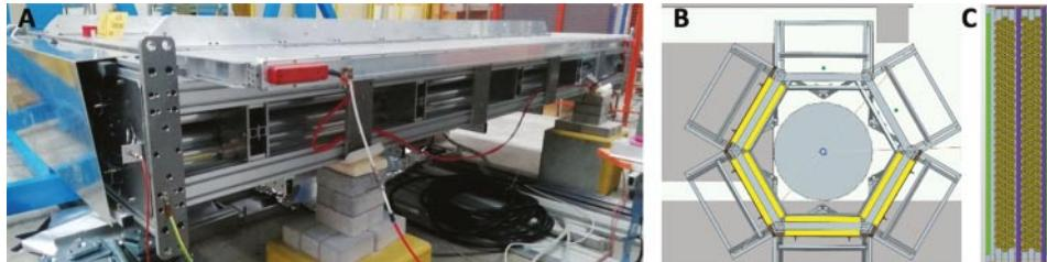
Fig. 6. – (A) Detector segment obtained by adding the INFN Muon Detector (upper part) to the drift tube module (lower part). (B) Detector positions. (C) Top view drawing of a six-layer drift tube muon detector module. Pictures from [15].
