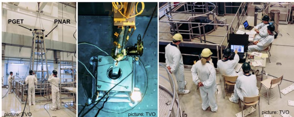
Fig. 7. – Left: the PGET and PNAR instrument at the top of their support structure before lowering into the spent fuel storage pool. Middle: A fuel assembly in measurement position. Right: Pool-side operation of the PGET and PNAR instruments.
