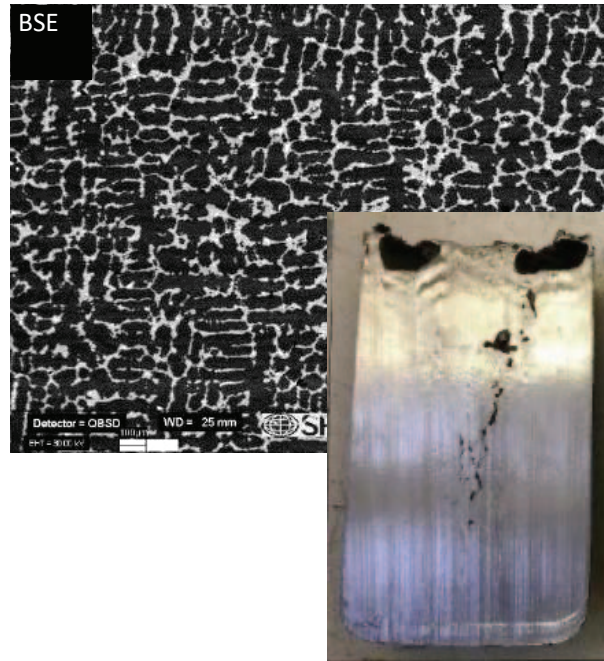
Fig. 3. – Cross section and microstructure of a melt processed ingot (provided by A. Duncan, SRNL).
