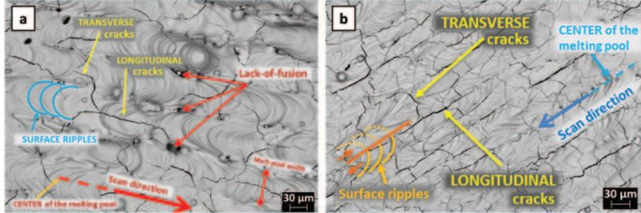
Fig. 1. – The crack network homogenously distributed on W [16] (a) and Mo [15] (b) manufactured by LPBF.
