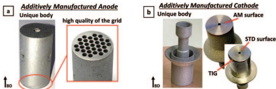
Fig. 3. – (a) The additively manufactured molybdenum anode and (b) the additively manufactured tantalum cathode.
