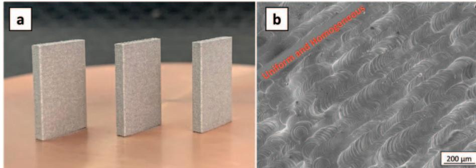
Fig. 2. – (a) The additively manufactured tantalum sample for process parameters tuning; (b) top surface morphology of the tantalum tag.
