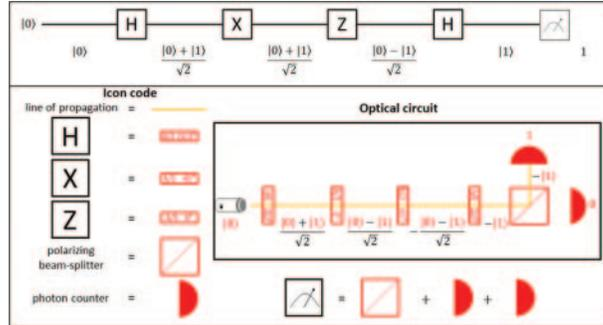
Fig. 2. – Top: an example of simple logic circuit proposed to students. Bottom: ideal realization of the circuit on an optical bench. For maximizing educational effectiveness, we introduce a color code (fig. 5) to identify visual elements pertaining to the polarization encoding, which are represented in red. For instance, half-wave plates are red rectangles with the caption  $\lambda/2$  and the angle of the slow axis.
