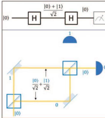
Fig. 4. – Top: an example of logic circuit. Bottom: its ideal implementation using spatial mode encoding.
