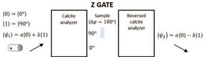
Fig. 1. – Idealized design of a Z gate on a polarization-encoded qubit.
