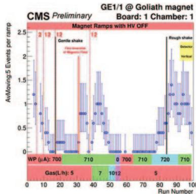
Fig. 3. – Evolution of the number discharges observed per magnet ramp. The discharge rate is computed using a moving average over 5 consecutive magnet ramps.
