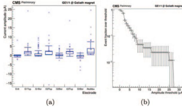
Fig. 2. – (a) Maximum current value observed per each discharge. The bins illustrate this value for each electrode and the maximum value observed among the 7 electrodes during each discharge event (AbsMax); (b) Fraction of discharges where the maximum current observed during the discharge event overcomes a given threshold value.
