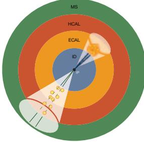
Fig. 2. –  $\mu$ LJ (lower-left cone) and  $e$ LJ (upper-right cone) inside the ATLAS barrel transverse plane. The outer circle represents the Muons Spectrometer (MS), the red circle the Hadronic CALorimeter (HCAL), the orange circle the Electromagnetic CALorimeter (ECAL), the blue circle the Inner Detector (ID). The black dot is the Interaction Point (IP), the yellow circles are energy releases, and continuous lines are tracks.
