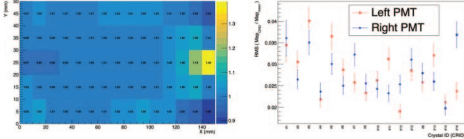
Fig. 1. – Left side: measured signal MPV variation map (with cosmic muons) taken with a PMT at  $x = 150$  and  $y = 25$  mm (MPVs are normalized to that measured in the centre). This map represents the mean one among the 16 crystals. Right side: RMS of the ratio bin to bin (75 values) between the map of each crystal and the mean one. Crystal ID (CRID) from 1 to 6 are mounted in the Flight Model (FM), 7 to 12 in the Qualification Model (QM) and the rest are spares.
