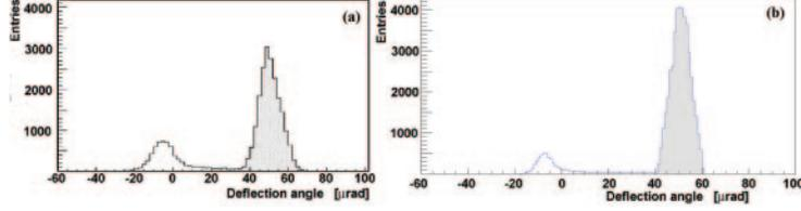
Fig. 1. – Deflection angle distribution for 400 GeV protons from UA9 data (left) [7], and Geant4 simulation (right).
