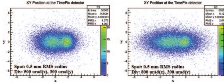
Fig. 3. – Beam spot at the TimePix3 plane for a detector to crystal distance of 2 m. Beam spot RMS size:  $\sigma(r) = 0.5$  mm; divergence:  $\sigma'(x) = 500\text{--}800$   $\mu\text{rad}$ .
