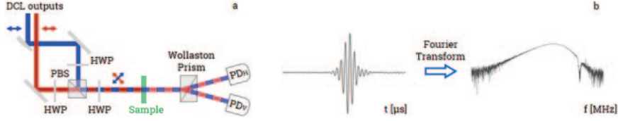
Fig. 1. – (a) Comb 1 (red) and comb 2 (blue) with their respective polarization states (red and blue double-sided arrows). (b) A typical interferogram recorded after the Wollaston prism and the associated Fourier-transformed spectrum in the RF range.
