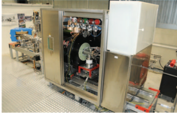
Fig. 1. – The Advanced Ion Source for Hadrontherapy at INFN-LNS in Catania.
