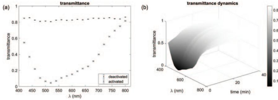
Fig. 4. – (a) Transmittance of activated and deactivated photochromic contact lens in the range under consideration, and whole deactivation dynamics in time (b).
