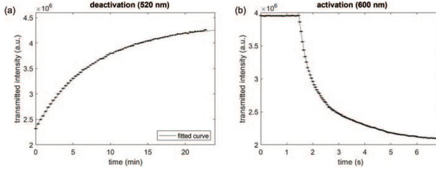
Fig. 3. – Examples of beam acquisitions in time for deactivation (a) and deactivation (b). Data refer to the energy integrated over a region of interest (ROI) of the camera including the transmitted beam (fig. 2(e)).
