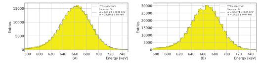
Fig. 2. -662 keV photoelectric peak of a  $^{137}$ Cs source, acquired with a Saint Gobain NaI:Tl, used to measure the energy resolution with the portable system (A) and with the standard one (B).
