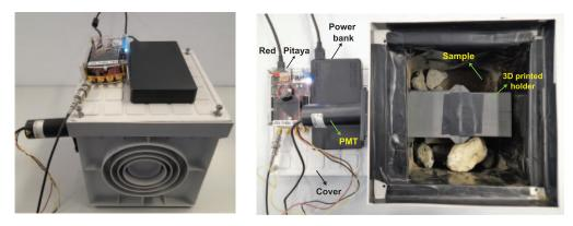
Fig. 1. – Left: the box with the detector inside, the *Red Pitaya STEMlab 125-14* and the power bank (20000 mA/h) on the top. Right: the inner part of the box. From left to right: the *Red Pitaya STEMlab 125-14* and the power bank placed on the lid of the box that contains the environmental sample and the 3D case with the photomultiplier tube and the CsI:Tl crystal.
