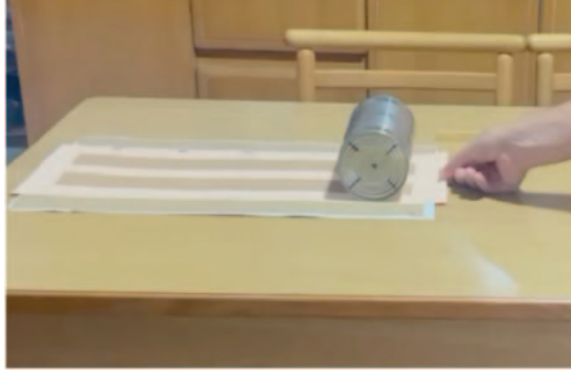
Fig. 3. – An accelerated conveyor belt can be replaced by a sheet of paper pulled from rest with acceleration \vec{a}_{O'} on a table. The food can is seen to roll as specified in fig. 1 when the paper is pulled.
