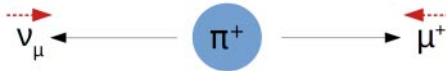
Fig. 2. – Decay of the positive pion in the rest frame of reference. The spin of the muon points toward the pion as the neutrino must be left-handed because of parity violation of the weak interaction.
