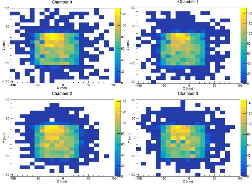
Fig. 4. – Occupancy plots for the four resistive MicroMegas tested under muon beam at the SPS in July 2023. The beam (large about 8 cm in xy direction) hit the central area of the chambers.
