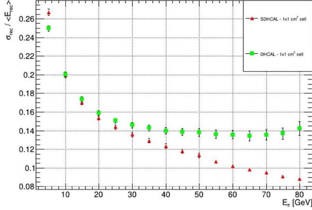
Fig. 3. – Comparison between energy resolutions obtained in the case of the digital readout, in green, and the semi-digital one, in red.
