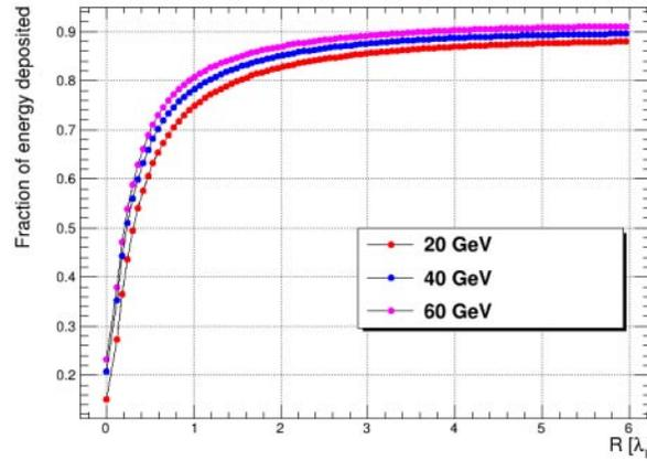
Fig. 2. – Lateral shower containment, expressed in terms of fraction of deposited energy, as a function of the cylinder radius in unit of nuclear interaction length  $\lambda_I$ , for three different values of the  $\pi^-$  energy. This plot is obtained with 100 layers.
