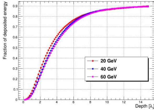
Fig. 1. – Longitudinal shower containment, expressed in terms of fraction of deposited energy, as a function of the depth in unit of nuclear interaction length  $\lambda_I$ , for three different values of the  $\pi^-$  energy. This plot is obtained with lateral surface dimension of  $1 \times 1 \text{ m}^2$ .
