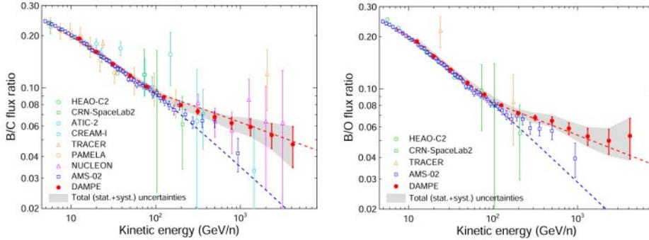
Fig. 4. – Boron-to-carbon (left) and boron-to-oxygen (right) flux ratios as a function of the energy per nucleon measured by the DAMPE instrument. The error bars represent the statistical uncertainty, while the shaded bands denote the total uncertainty (sum in quadrature of the statistical and systematic uncertainties). More details in ref. [10].
