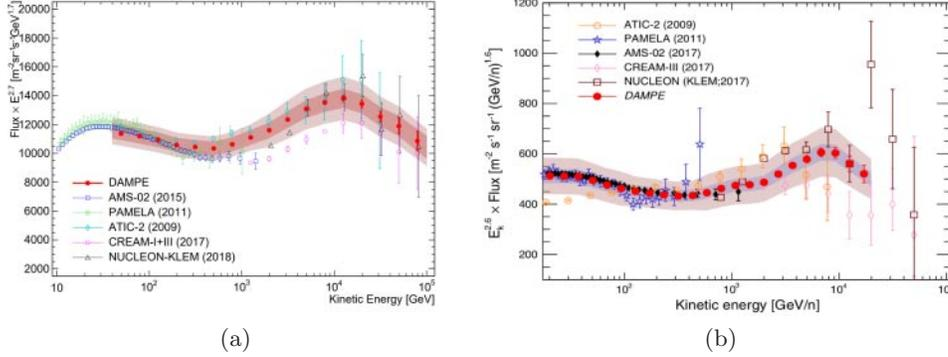
Fig. 2. – Proton (a) [4] and helium (b) [7] energy spectra measured by the DAMPE instrument, compared with the results of the previous experiments. The error bars represent the statistical uncertainties, while the inner and outer bands denote the systematic uncertainties from the analysis and the total systematic uncertainties.
