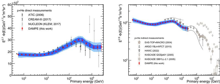
Fig. 3. – p+He spectrum measured with the DAMPE detector, compared with direct (left) and indirect (right) measurements. The statistical uncertainties are represented by error bars, while the continuous bands represent the systematic uncertainties on the analysis (inner band) and the total systematic uncertainties (outer band). More details in ref. [9].
