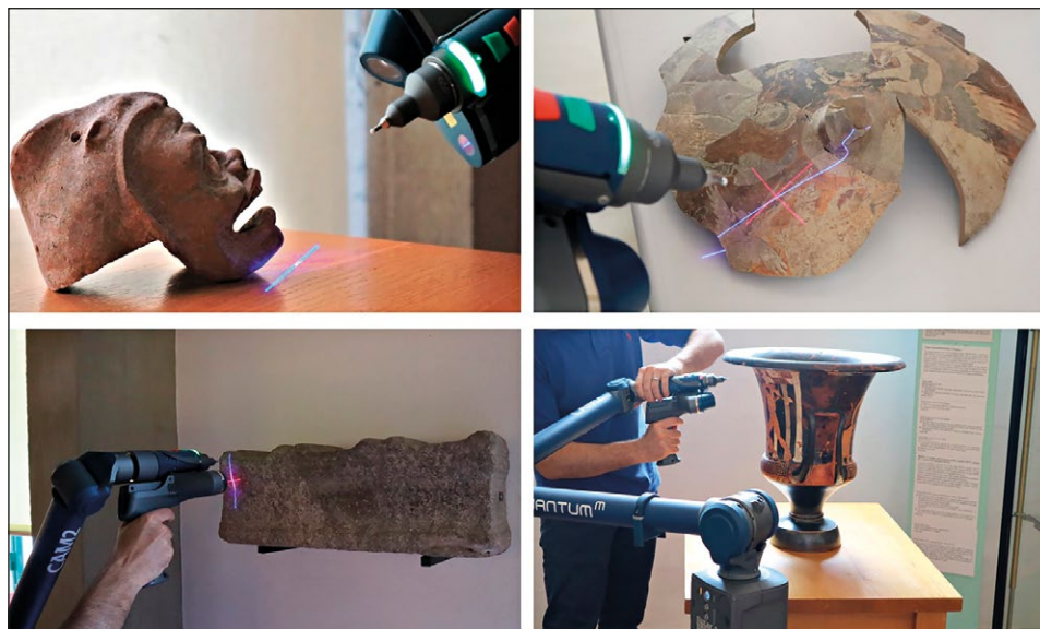
Fig. 3 – Laser arm scanning in progress.
