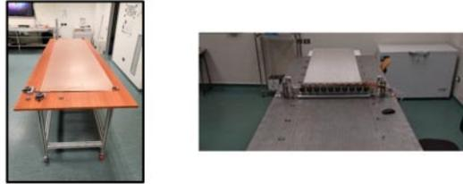
Fig. 3. – Left: the stand table used to measure the lateral dimension of the panel. Right: ten analog linear probes measure the thickness of the panel with respect the granite table with a granularity 70x70 mm and a precision of 10  $\mu$ m.
