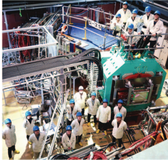
Fig. 1. – A picture of the S-2S spectrometer installed at the K1.8 beam line area of the J-PARC hadron hall. It consists of the QQD magnet system.
