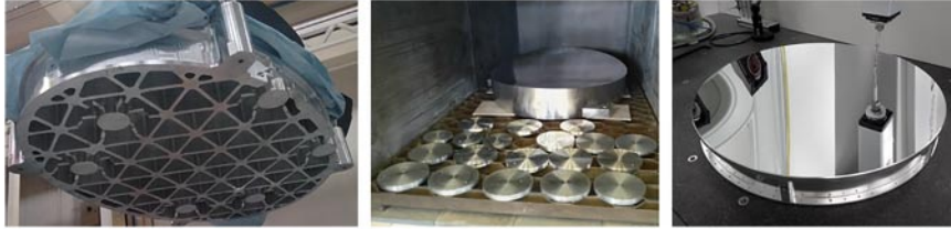
Fig. 4. – (Left) Photo of the back of the Engineering Model (EM) mirror which shows the triangular pattern lightening. (Center) Photo of the Pathfinder Mirror (PTM) together with 150 mm diameter samples inside an oven to carry out a hot thermal treatment. (Right) Photo of the 0.7 m diameter mirror after having carried out a diamond turning. Credit: Italian Telescope Assembly Team.
