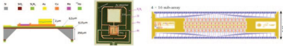
Fig. 2. – Left: side and top view of the Holmes detector. Right: array of TES organised in 4 rows of 16 TES each used in Holmes [5].
