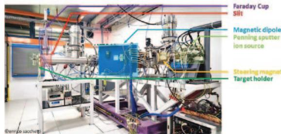
Fig. 3. – Picture of the current implanter with the components highlighted.
