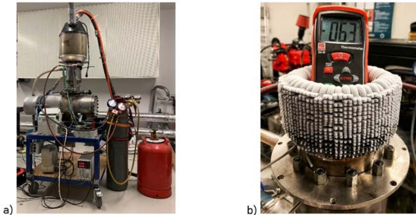
Figure 1. a) The \beta -Stirling-engine with connected helium and propane reservoirs and exhaust pipe ready for operation as a heat engine in the engine laboratory at Western Norway University of Applied Sciences; b) The exposed and ice-covered heat exchanger at the top of the engine at -63^{\circ}\text{C} while cooling down in cooling mode.
