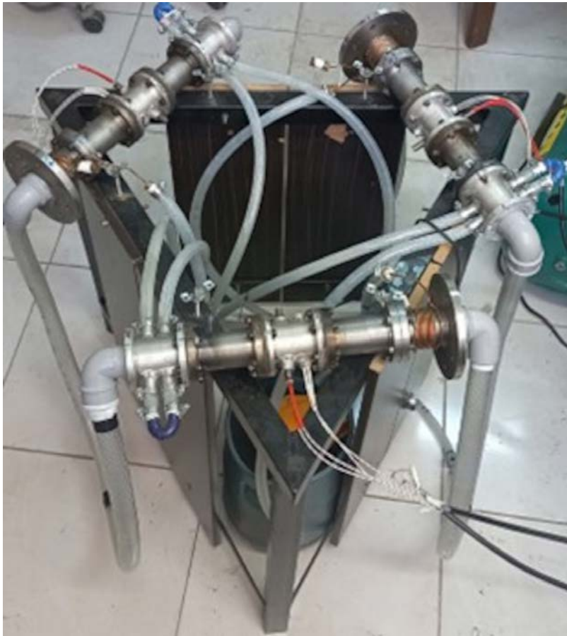
Figure 10. The developed three-stage double-acting Fluidyne Stirling oscillator.
