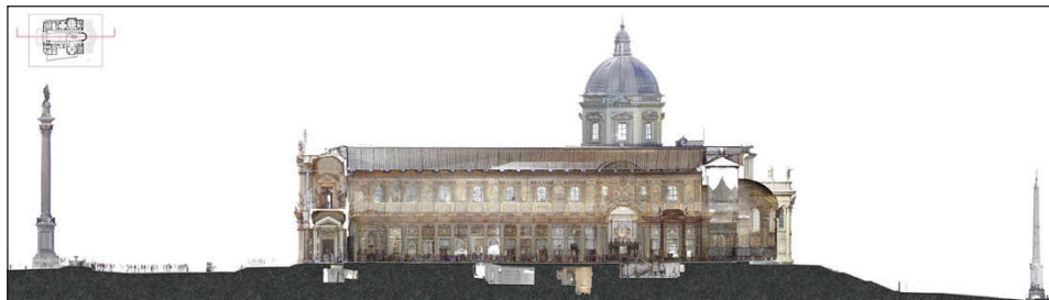
Fig. 3 – Longitudinal section-laser scanner point cloud.
