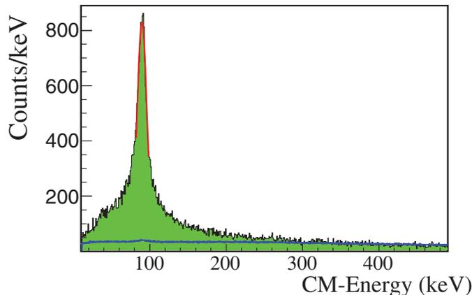
Fig. 1. – The  ${}^8\text{Be}_{g.s.}$  resonance measured in 2- $\alpha$ -particles coincidences. The red line is a Gaussian fit of the resonance. The blue line is the background computed with the event mixing technique.
