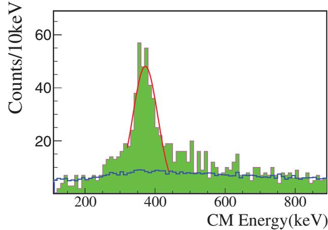
Fig. 2. – The Hoyle state resonance measured in 3- $\alpha$ -particles coincidences. The red line is a Gaussian fit of the resonance. The blue line is the background computed with the event mixing technique.
