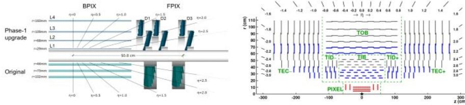
Fig. 1. – Layout of the CMS tracker. The figure on the left, the layout of the pixel detector, is from [4], the figure on the right, the overall layout of the tracker, is from [2].
