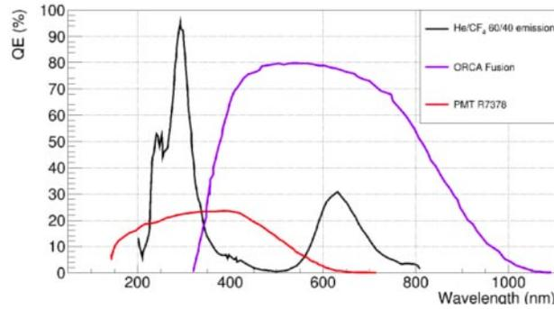
Fig. 3. – The superimposition of the electro-luminescence spectra of the He:CF<sub>4</sub> gas mixture in black, the quantum efficiency of the Hamamatsu Orca Fusion camera in violet and the Hamamatsu PMT in red.
