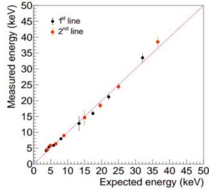
Fig. 4. – The linearity response of the LIME prototype.
