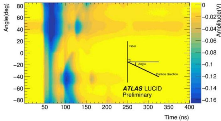
Fig. 5. – Signal generated inside the fiber by a beam of 200 MeV electrons as function of the beam direction [9]
