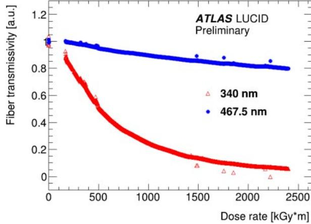
Fig. 3. – Fiber transmissivity loss at 340 nm (red) and at 467.5 nm (blue) as function of the absorbed dose [9].
