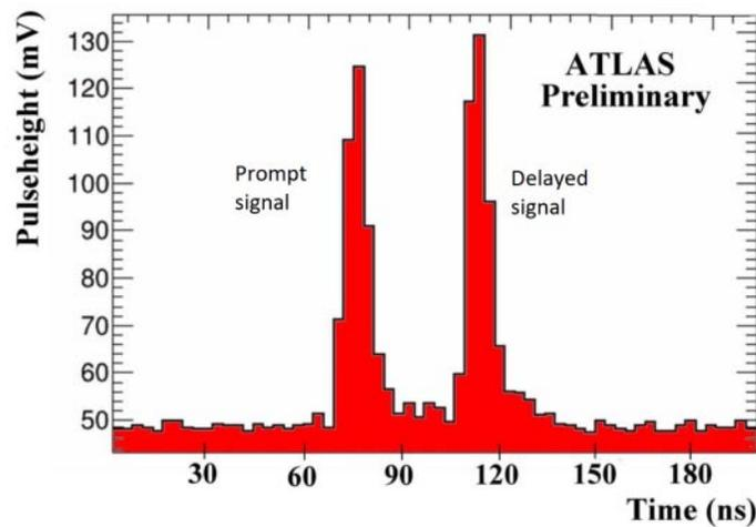
Fig. 2. – Example of a signal generated by an LED inside the PMT. LED light is divided in two part: the first one goes directly to the PMT (prompt signal) while the second one goes through the fiber (delayed signal) [8].
