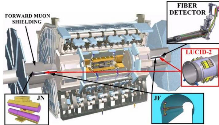
Fig. 1. – Design and placement of LUCID-2 and LUCID-3 prototype (JF, JN and Fiber) inside the ATLAS experiment [7].
