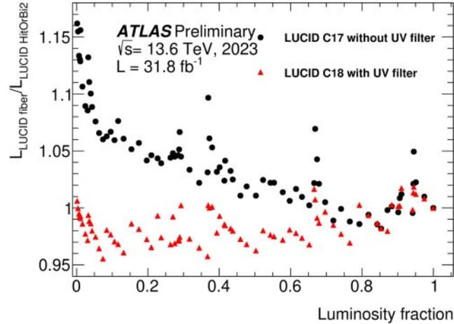
Fig. 4. – Fill by fill ratio of luminosity measured by the both fiber prototypes (without UV filter black dots, with UV filter red triangles [10]).
