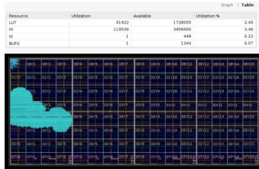
Fig. 8. – Occupancy of the FPGA resources during the preliminary studies for the pattern-matching algorithm. This test only includes the matching logic between incoming data and patterns. The priority encoder selecting the best muon candidate is not included.
