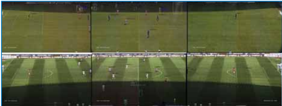
Global view of the field of game observed from the 6 TVcameras from opposite sides; The system has automatically determined the position of all the players in the field of game and identifies the player that makes the launch of the ball.
