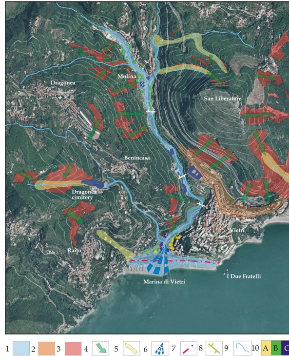
Figure 5: Geological effects and damage pattern induced by the 1954 flood event. (1) Overflowing area, (2) mud deposits, (3) evidence of past denudation, (4) landslide phenomena, (5) channelled debris flow, (6) alluvial fan, (7) shoreline before 1954 event, (8) temporary dam, (9) drainage network, (10) damage categories: (A) heavy, (B) medium, (C) light [5].
