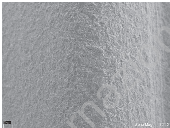
Figure 7 - SEM visualization of the Micro Rough Surface® regularly distributed (721x magnification).
