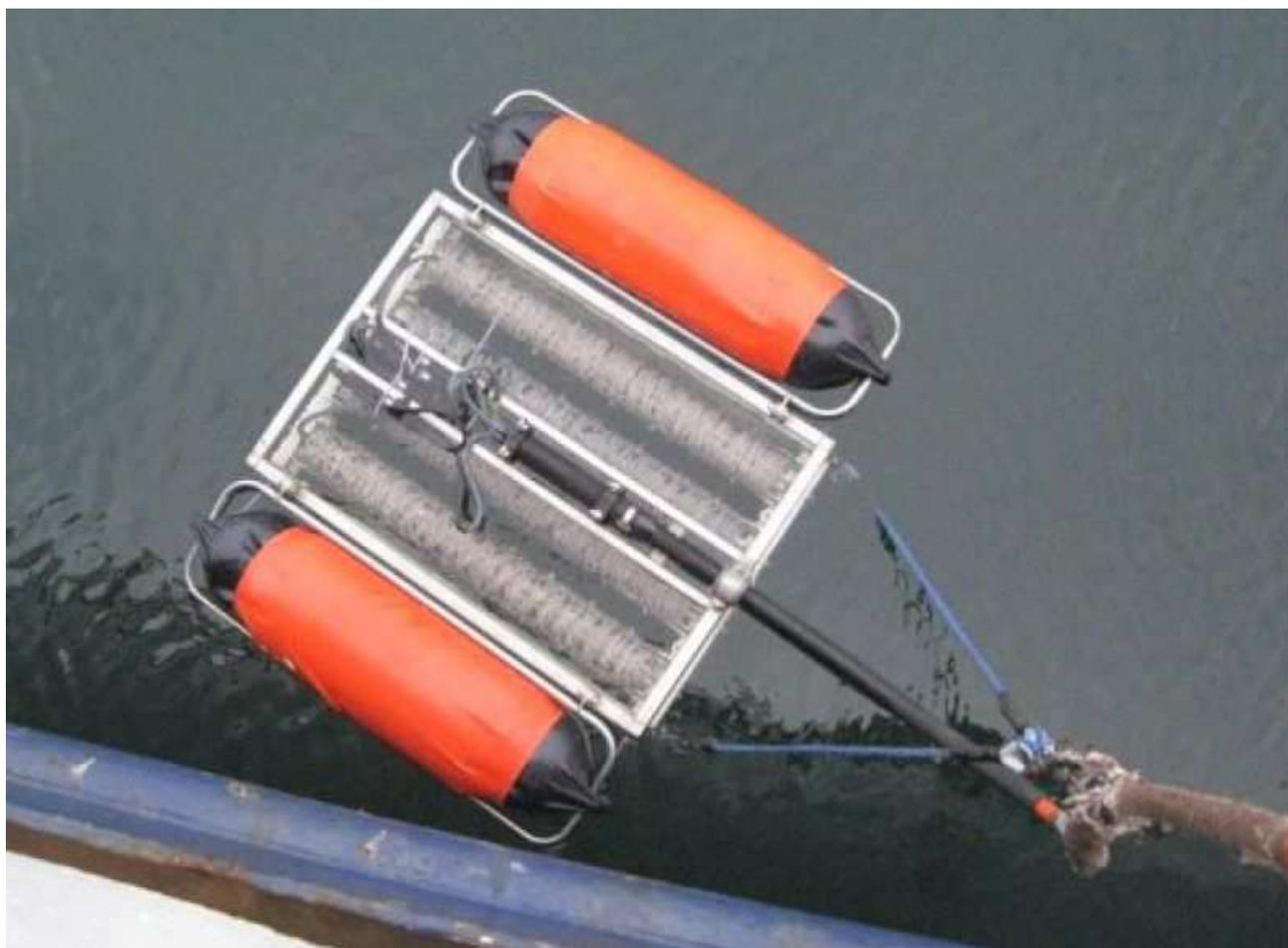
**Figura 7 - Geo-Source 400 Marine Multi-Tip Sparker.**
