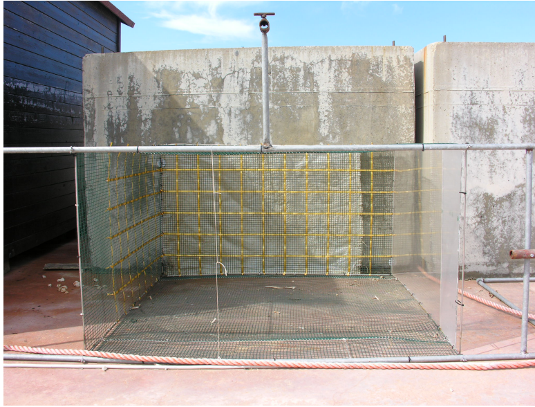
Figure 16. Grids affixed on the sides of the sea cage
