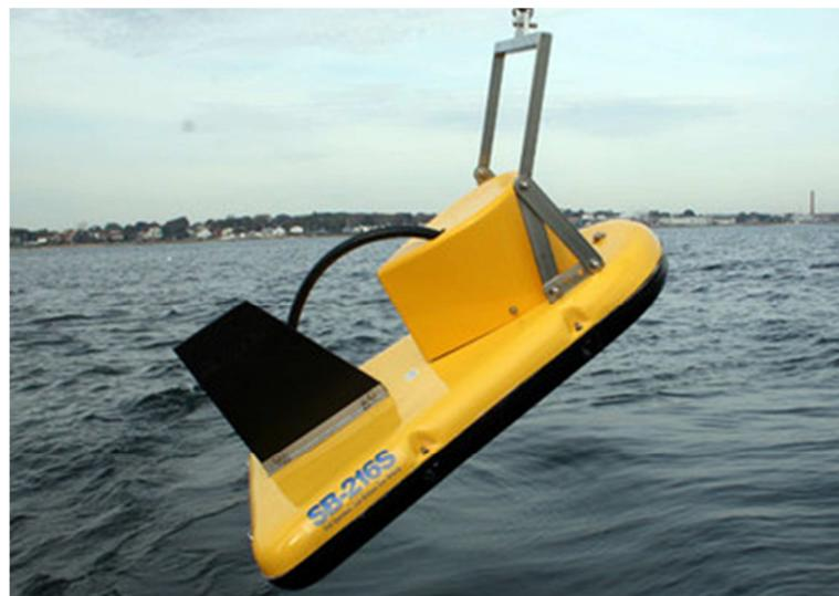
Figura 18 – Sub-bottom profiler Edgetech 3100 modello 216S
